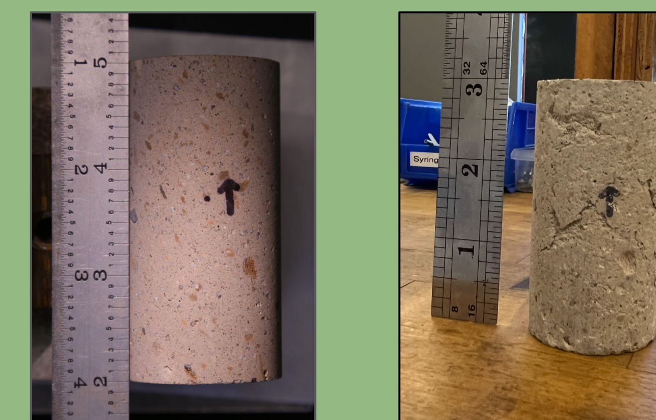
Pre-(left) and Post-Failure (right) of sample RORD22_13_1 under 50 MPa confining pressure.
